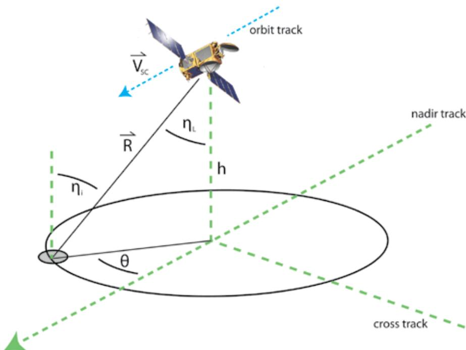
Figure 5. Measurement geometry for a scanning scatterometer system. Wide-swath coverage is achieved by scanning a pencil-beam footprint at a fixed incidence angle,  $\eta_i$ , through an azimuth scan angle ( $\theta$ ) range of  $360^\circ$ .
